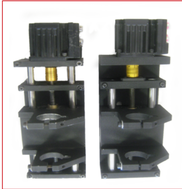
Rev 2 Lifter Station Rev 3 Lifter Station
